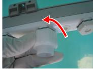
2. Wipe off the electrode probe and around it with a cotton swab immersed in alcohol.
